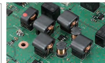
Transformer feedback RF Amp
